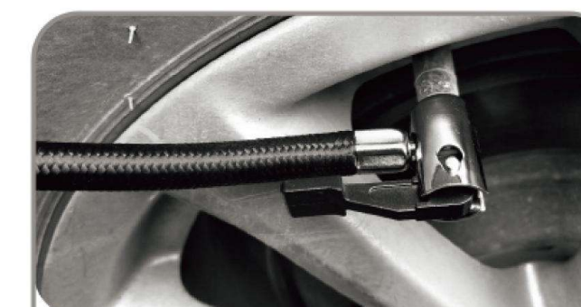
3the inflatable port is connected to the tire air nozzle
